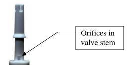
Figure 16: Location of valve orifices
