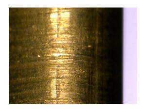
Figure 5: Bead of an Aluminum can magnified 88X showing eyelashing
