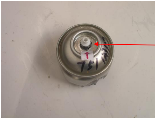
Figure 14 - From customer showing Damaged Seal bead
