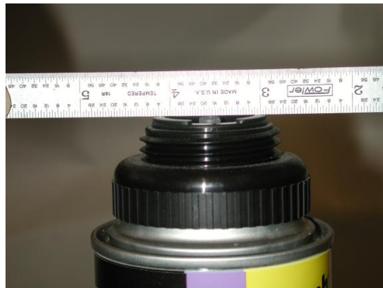
Figure 8 - Tip of valve stem with respect to top of collar
