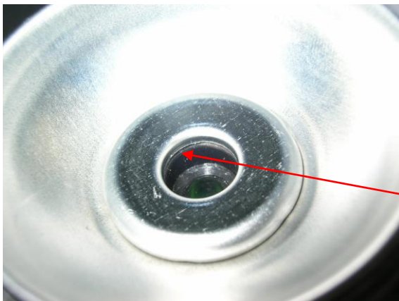
Figure 18 – No Clearance for the Bead of the Rubber Seal
