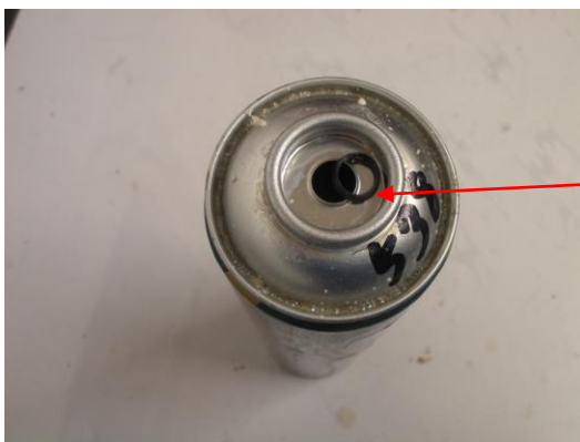
Figures 15 - From Customer Show Bead Completely Torn Off and Stem and Seal Pushed into Can
